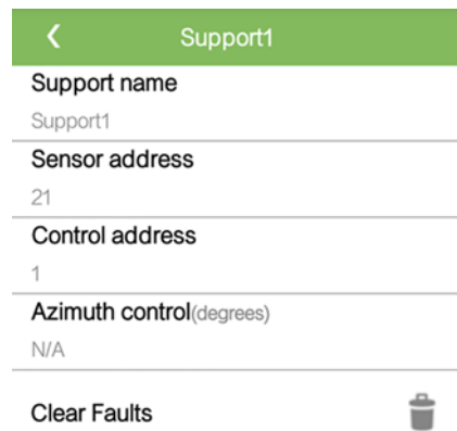
Figure 7-15 Setting parameters of a single support
