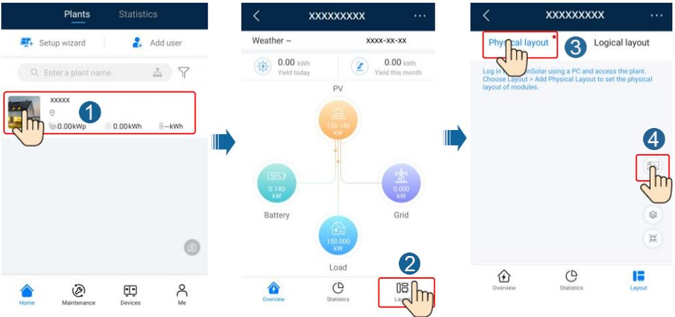
2. Log in to <https://intl.fusionsolar.huawei.com> to access the WebUI of the FusionSolar Smart PV Management System. On the **Home** page, click the plant name to go to the plant page. Select **layout**. Choose **Generate layout**, and create a physical layout as prompted. You can also manually create a physical location layout.
